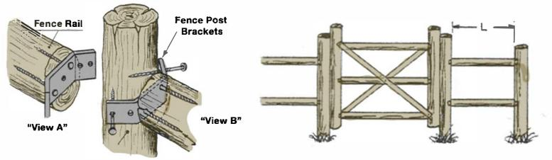
Cut fence rails to match length of space "L" between fence posts, as illustrated. Using spiral or ring shank nails, attach fence post brackets to ends of rails as illustrated, View "A". Two or three nails may be used as best suited.
